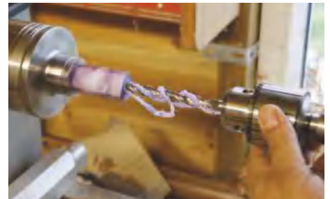
▲ Pic.1 Drill the blank with the correct diameter hole to suit the kit
